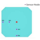
(c) Cavity geometry and pressure sensor location
