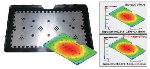
Fig. 1 The warpage results of the original material
